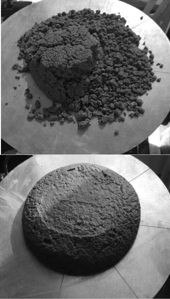
Figure 4. The use of water-reducing admixtures can aid in establishing equivalent flow to facilitate sample casting at a range of binder compositions and w/b. Images above show flow test results for same binder at same w/b, without (top) and with (below) HRWR. [Photo courtesy of Behnaz Zaribaf.]
