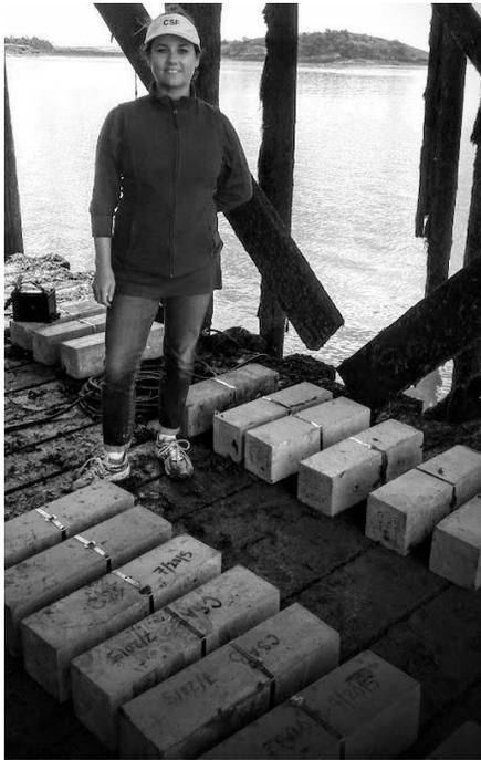
Figure 2. The first author with ACM concrete prisms placed at the US Army's outdoor field exposure site in Treat Island, Maine in August 2015.
