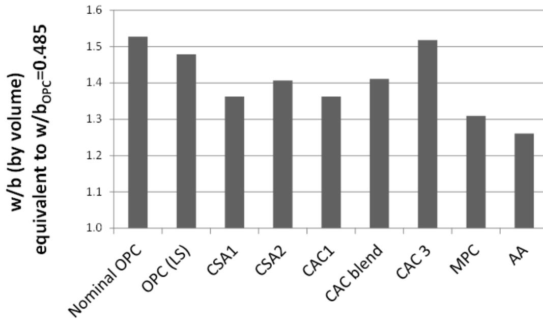
Figure 3. Comparison of initial w/b ratio by volume for pastes produced from a range of alternative cementitious materials at a 0.485 ratio by mass show large differences in water-filled porosity.
