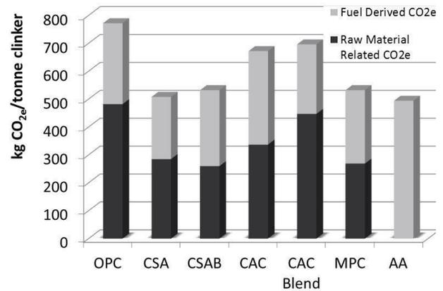
Figure 1. Comparison of embodied carbon dioxide between portland cement (OPC) and various ACMs, assuming a 1:1 by mass usage rate. Based upon [5].
